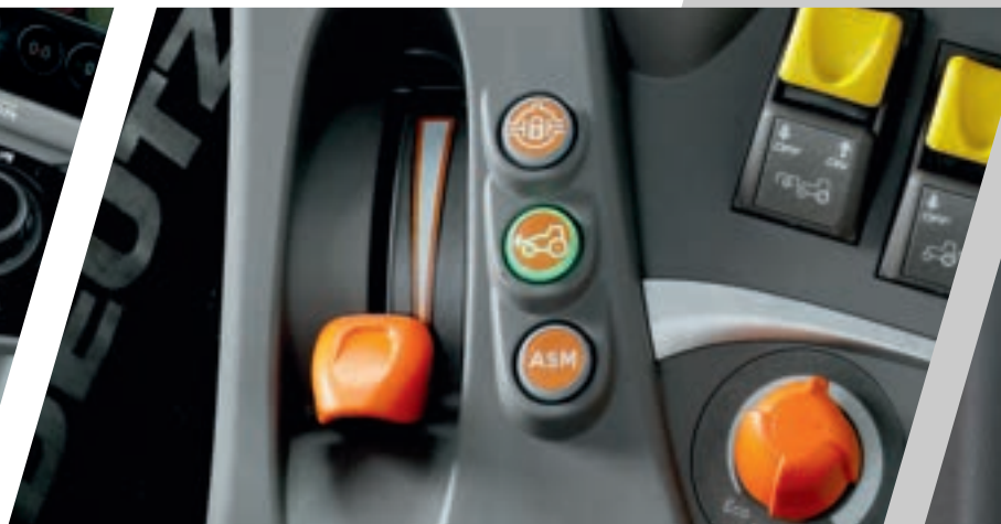
> Electro-hydraulically operated all-wheel drive and differential lock with ASM button and independent hand throttle.
